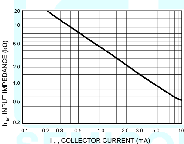
I_C , COLLECTOR CURRENT (mA) Figure 11. Input Impedance
